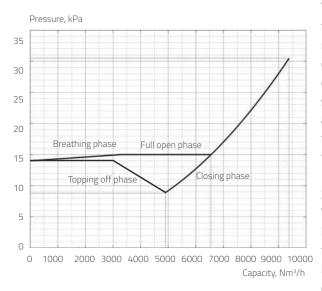
The patented PV-VOC pressure/vacuum valve is designed to optimize the VOC performance. Using fluid dynamic simulation software in connection with testing, we have achieved a performance that benefits all stages in the operation of an oil tanker. This includes filling, topping, breathing or VOC savings in accordance with the VOC management procedure required by IMO/MSC/ Circ.680.
