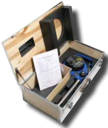
**Special tape protection** to protect the tape from inadvertent cuts by closing the valve while the sensor is inside the tank. This mechanical safety device prevents damages on tape and reduces repair costs.
